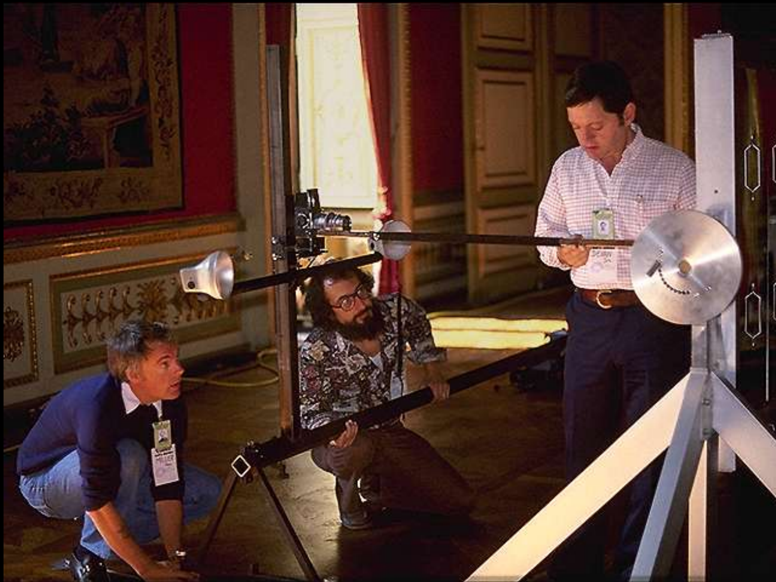
Vern Miller, Sam Pellicori and Don Devan calibrating camera rail system
