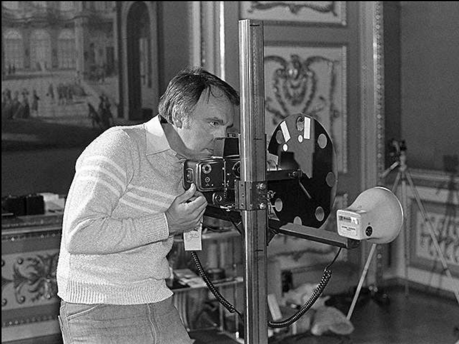
Vernon Miller using Hasselblad camera mounted on Camera Support Rail with rotating wheel mounted in front of the lens housing the B/G/R filters
