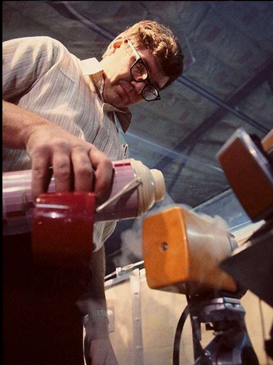
Steve Baumgart (1 st slide) and Tom Haverty add liquid nitrogen to their thermographic instruments
