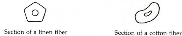
(Fig. 3). Raes' comparison drawings between linen and cotton. Note the pentagonal shape of linen compared to the flattened ribbon- like shape of cotton. (Illustration adapted by Paul C. Maloney taken from Shroud Spectrum International , Vol. IX, no. 38-39, p. 6).
