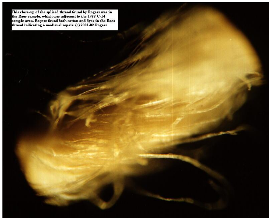
(Fig. 7) Photomicrograph of the Rogers' spliced thread. (Photo courtesy of Barrie Schwartz). (See also Appendix I below: Ray Rogers' e-mail regarding the splice).
