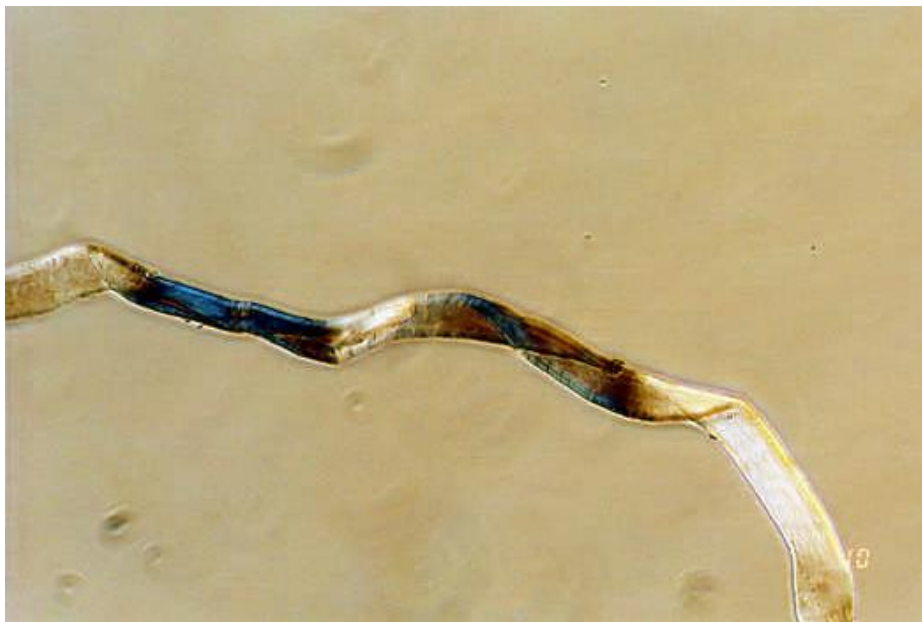
(Fig. 4). Brown's discovery of a cotton fiber removed from inside the frayed end of Raes thread R14. Note the lack of any encrustation. It was protected by the surrounding linen fibers. Light micrograph taken by John Brown at 315 X magnification. (Brown's Fig. 4).
