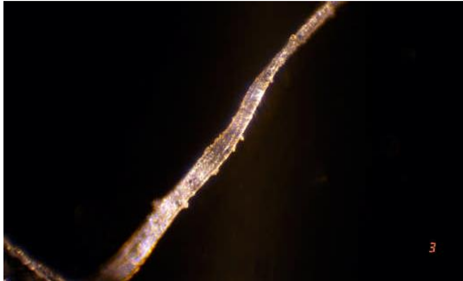
(Fig. 5). Light micrograph of the cotton fiber that wrapped the outside surface of Raes yarn no. R14 showing the coating of encrustations. Light micrograph, taken by John Brown at 315X. (Brown's figure 5)
