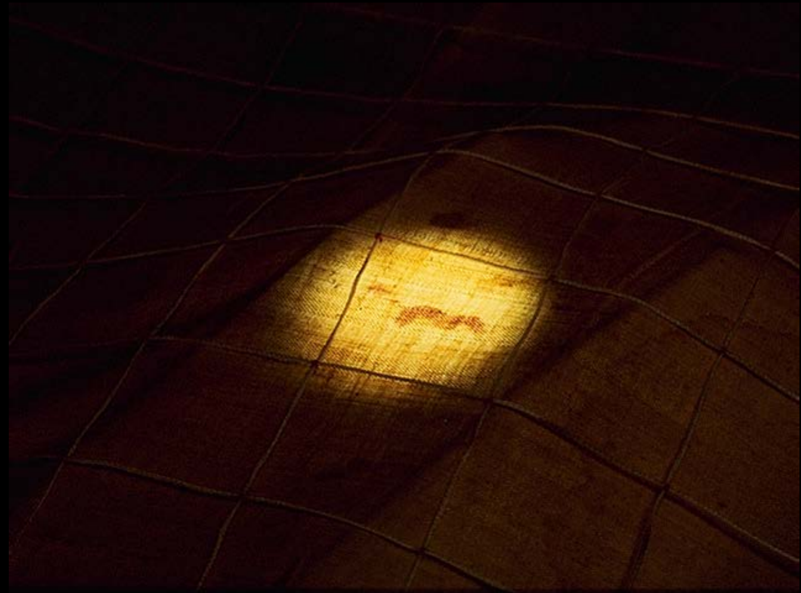
Prof. Giovanni Riggi's endoscopic camera focusing light transilluminates the #3 bloodstain on the forehead, revealing higher density in blood areas
