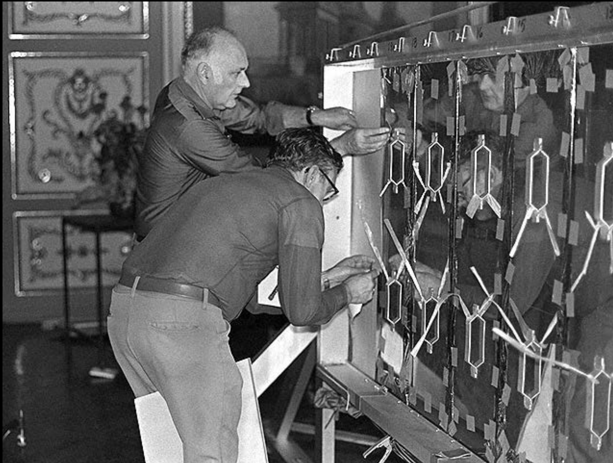
William Mottern and Ronald London remove the steel panels via the rear of the Shroud Examination Table to allow for x-rays to be taken of the cloth
