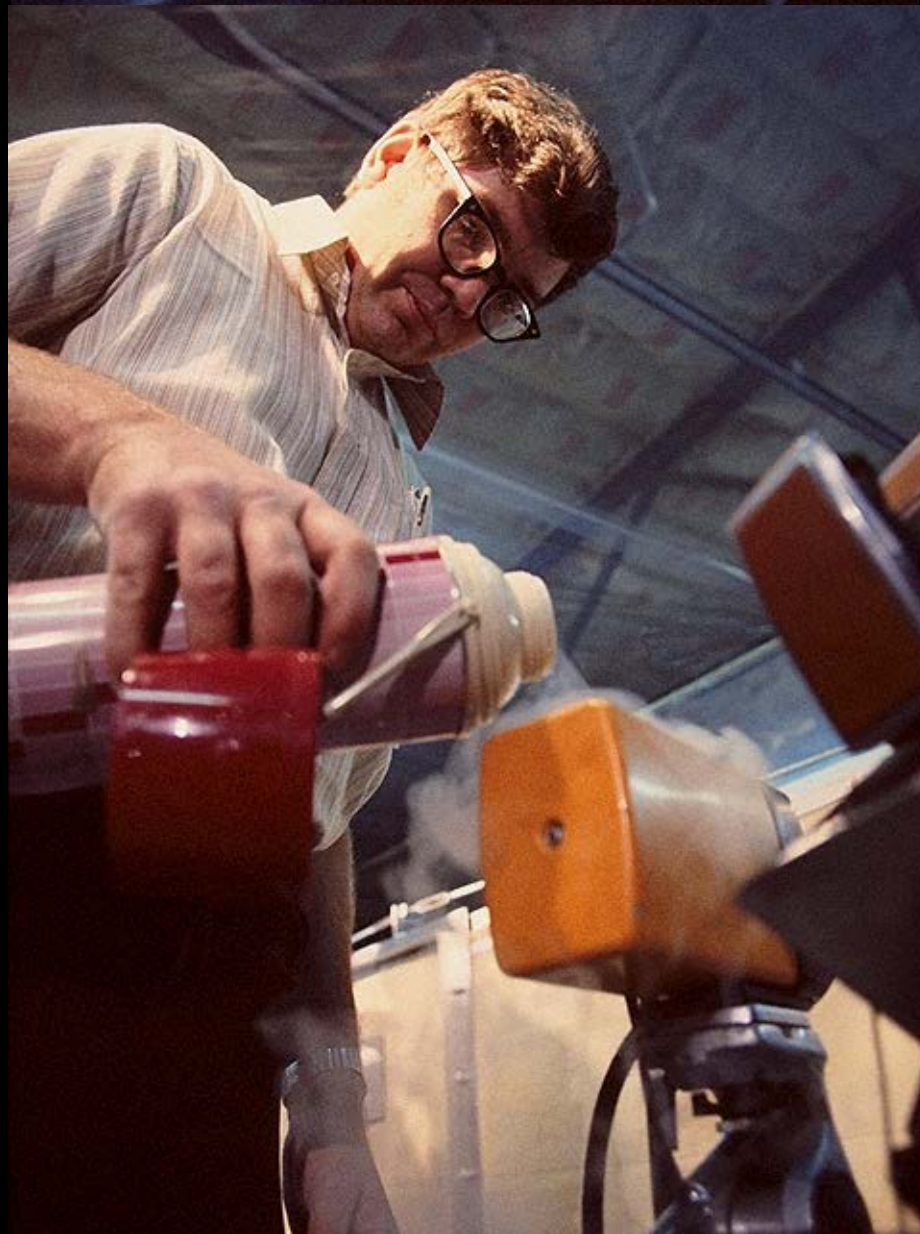
Steve Baumgart (1 st slide) and Tom Haverly add liquid nitrogen to their thermographic instruments
